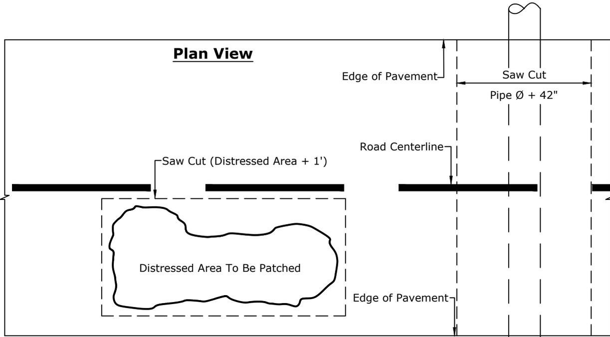
**Typical Pavement Repair Patch**
